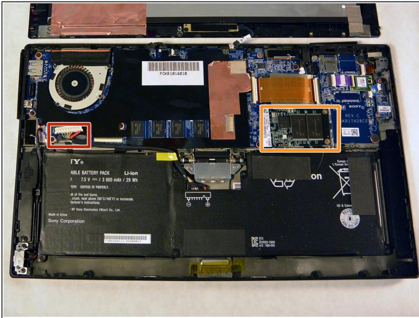
**⚠** Unplug the battery connector located beside the fan.
