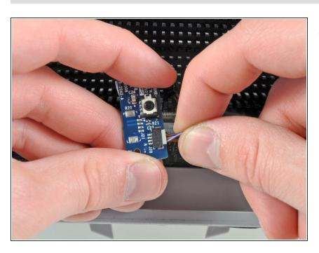
Disconnect the second IR board and remove it from the iMac.
