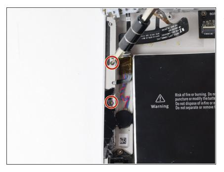
Remove the two 4 mm T3 Torx screws.
