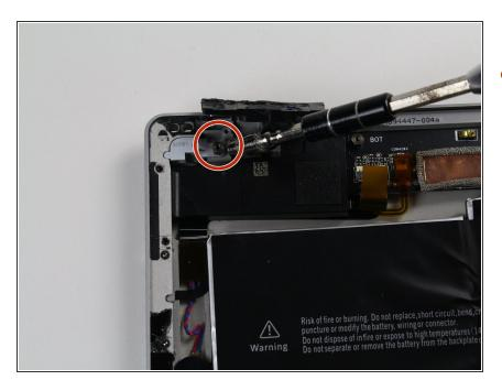
Remove the nut with the 4mm nut driver.
