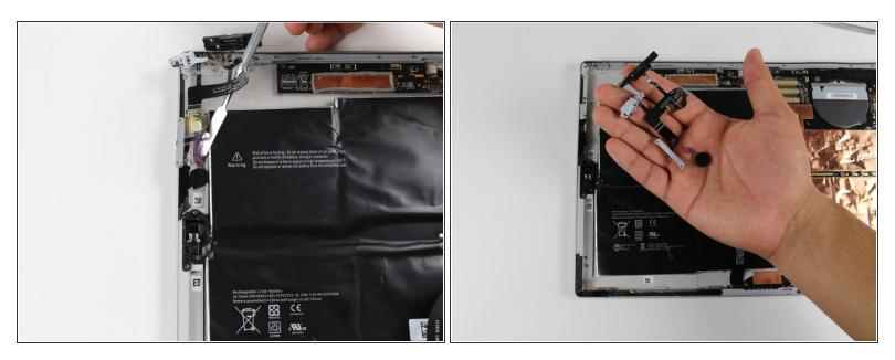
• Finish removing the headphone jack using the metal spudger.
