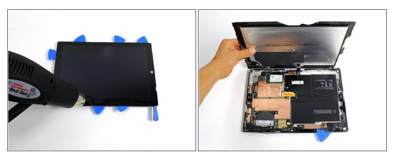
Lift the screen up carefully so that no wires are torn.
