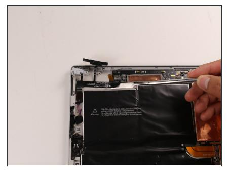
Use the metal spudger to remove the black ribbon wire from the device.
