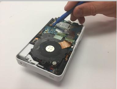
• Using the plastic opening tool, disconnect the three connectors from the motherboard.
