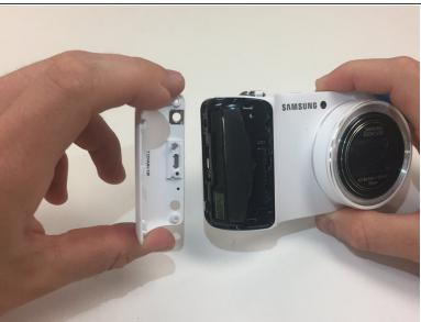
Use plastic opening tool to remove the cover on the non-lens side of the camera.
