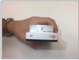
Remove all seven 4 millimeter long screws using the PH000 screwdriver bit.
