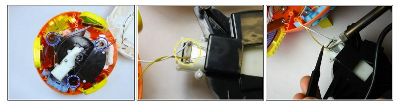
• Remove the motor by lifting it out of the shell, and find the attached wires at both ends: the circuit board and the motor itself. Use the soldering iron to remove the existing attachments by heating the solder joint with the solder iron tip while pulling on the wire.
