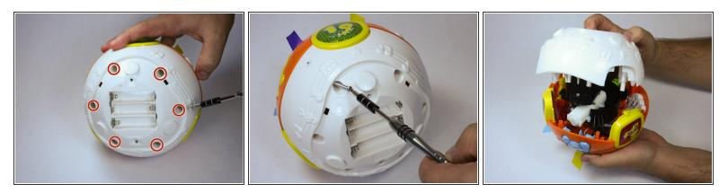
Remove 6 screws in order to pop off the outer shell and reach the inside components.
