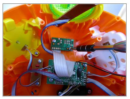
Unscrew the two screws to the power switch located beside the circuit board
