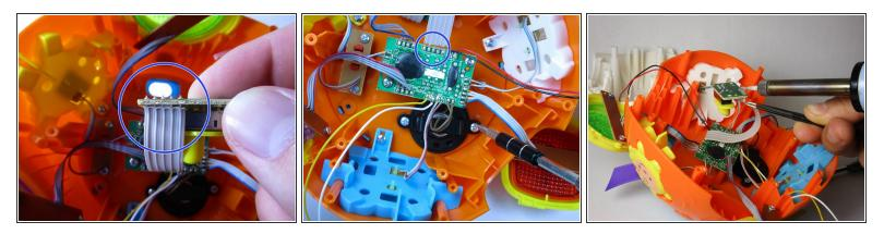
• Remove the existing attachments at both ends of the wires with the soldering iron. Heat the solder joint with the solder iron tip and pull the wire.
