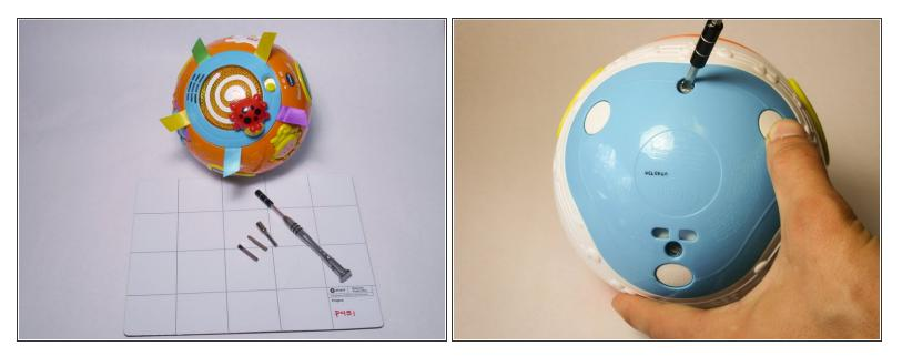
• There are two screws that require a 4.0mm flat head screwdriver. Twist them counter clockwise to remove. When you remove them they stay contained within the blue outer case.
