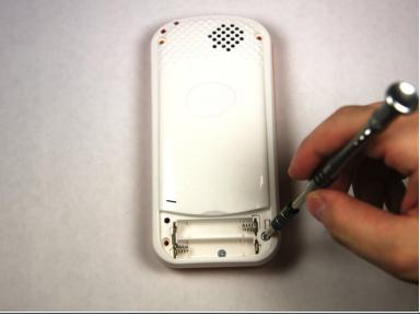
• Remove 4 13.8mm screws holding the device back using a Phillips #1 screw driver.
