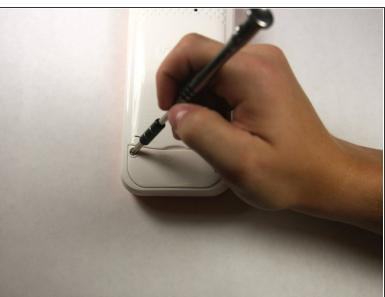
Using a Phillips #1 screwdriver, remove the 4.8mm screw on the battery cover by twisting the screwdriver counter-clockwise.
