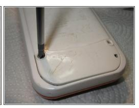
when reassembling, align the notch on the battery panel with the slot on the phone.
