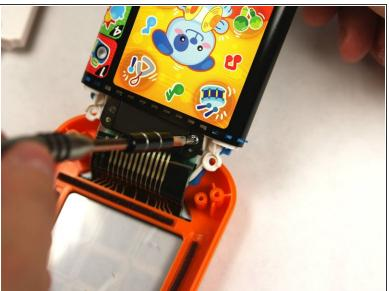
• Remove the two 7.5 mm screws with a Phillips #0 screwdriver.
