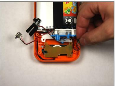
Remove the two buttons, noting how wires are placed for reassembly.
