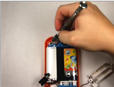
Remove four 7.5mm screws with a Phillips #0 screwdriver.
