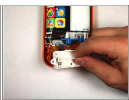
Remove a single 4.8 mm screw with a Phillips #0 screwdriver and lift away the battery pack being careful of the wires.
