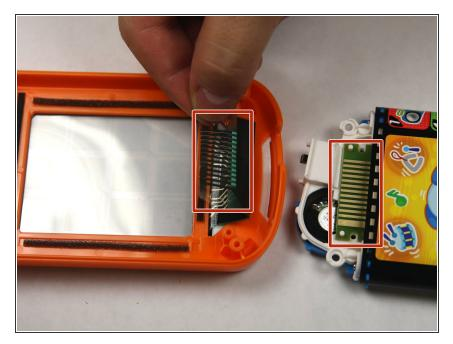
With the connector removed, clean both of the boxed sections with rubbing alcohol on a cotton swab.
