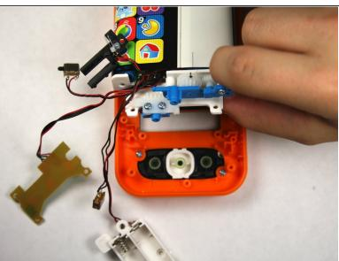
Lift the assembly to gain access to the connection point under the assembly.
