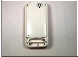
Remove the two AAA batteries by pulling on one end of the battery and lifting it straight out.
