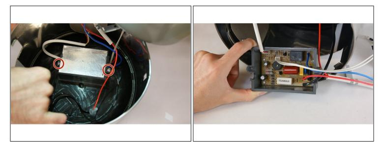
Using a Phillips head screwdriver, size PH2, remove the screws from the control module to expose wired connections.
