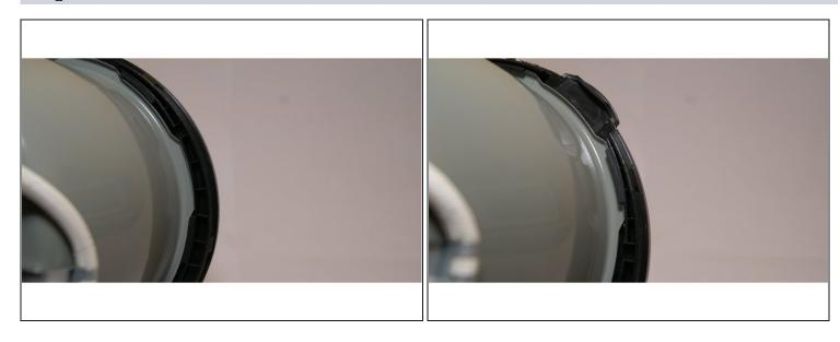
• Next, you must remove the upper black trim which is connected to the inside liner with tabs. To do this you must hold the interior walls still, while rotating the trim so that the tabs line up with the slots. (tabs cannot be seen at this point, pics are to give you an idea of what you cannot see inside the device)
