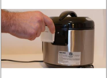
• The first step is removing the condensation catcher in order to reach the control panel. We do this by pinching the condensation catcher as shown, on both sides and pull the condensation catcher away from the cooker.
