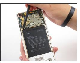
Use a spudger to detach the ribbons connected to the motherboard using an upward prying motion.
