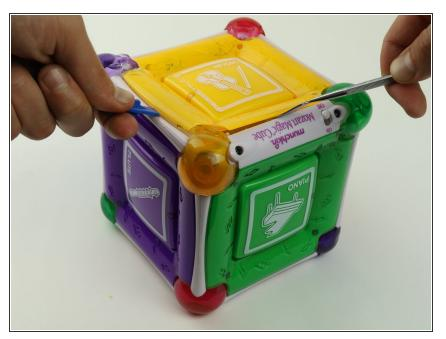
• Starting with the yellow face, insert the metal spudger between the yellow face and the white frame, prying the frame apart.
