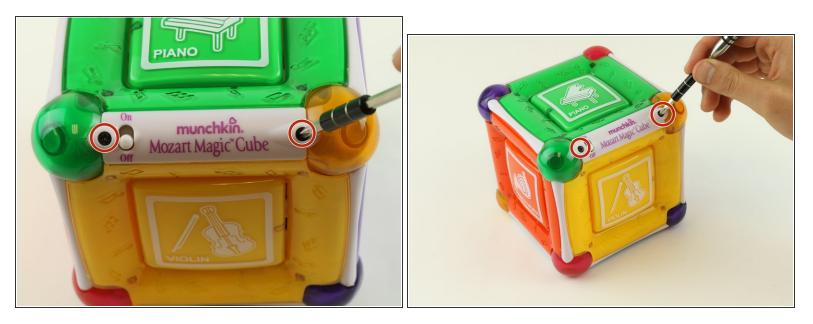
• Remove two 6 mm Phillips #2 screws on either side of the On/Off Plate.
