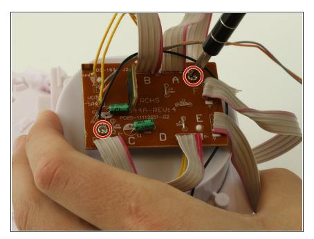
Remove two 6 mm Phillips #2 screws holding down the main motherboard to plastic frame.
