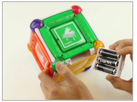
• Gently pull out the battery cartridge and if needed, replace the batteries with 3 AA alkaline batteries.
