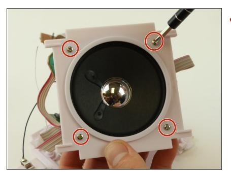
Remove four 6 mm Phillips #2 screws that hold down the speaker to its plastic frame.
