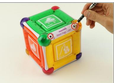
Remove two 6 mm Phillips #2 screws on either side of the On/Off Plate.
