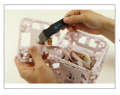
Flip the frame over so that green motherboard over so that the LED is face down and the brown side of the motherboard is face up using the Jimmy to remove the glue connecting the motherboard to the white frame.
