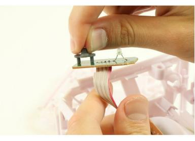
To remove the button use your fingers or forceps to remove the gray rubber button piece on the green side of the motherboard.
