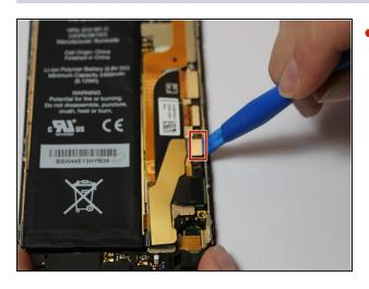
Disconnect the battery connection cable by using the plastic opening tool and applying light pressure upwards on the cable.
