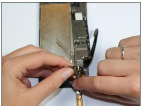
• Carefully lift up the motherboard and using the spudger pry camera from the camera holder
