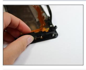
• Lift off bottom plastic piece with flat antenna cables
