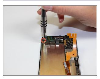
Unscrew the 3mm screw located on the top left side of the phone with a flat head
