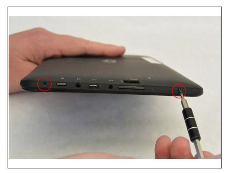
Remove the two Phillips #00 screws from the bottom of the case.
