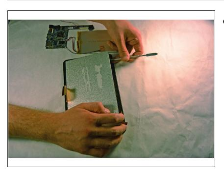
Using the metal spudger, pry the display from the screen.
