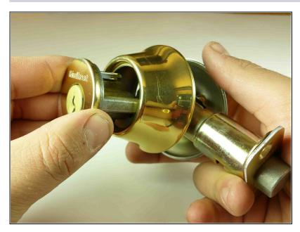
• Remove the cylinder assembly from the lock assembly.
