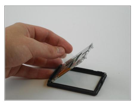
Finally, remove the LCD screen by grabbing the clear plastic tab and lifting it carefully. To reassemble your device, follow these instructions in reverse order.
