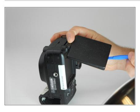
Using a plastic opening tool, carefully pry off the back cover of the LCD.
