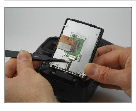
Using the tweezers, carefully disconnect the rear connector by pulling it away from the screen.
