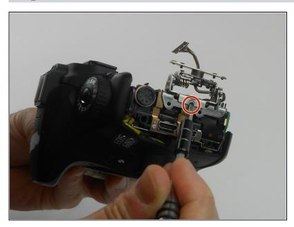
Remove one 2.8 mm Phillips #PH00 black screw on the side of the swivel assembly by using the PH00 screwdriver.
