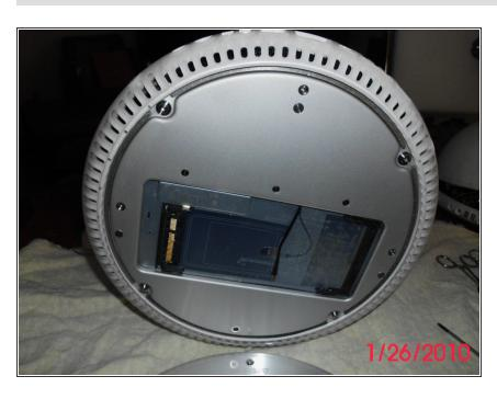
Here the plate has been removed exposing the slot for the Airport Card and User added RAM slot.
