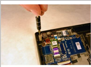
Using the Phillips #000, remove the two 3 mm screws.
