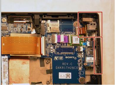
Once the battery is disconnected, locate the audio jack.
