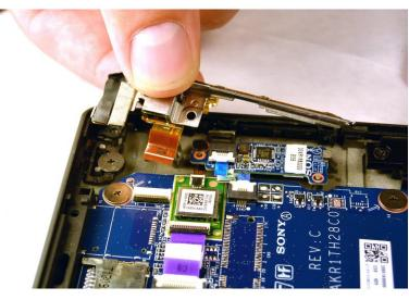
Disconnect the audio jack connector and remove the entire audio jack power volume button board assembly. To reassemble your device, follow these instructions in reverse order.
