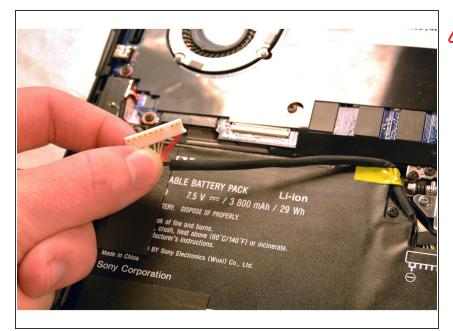
After removing the screen, disconnect the battery from the motherboard to avoid shock or the shorting of circuits.
