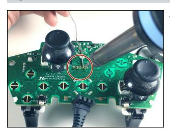
Re-solder the four nodes (left to right) with the soldering iron and soldering wire.
