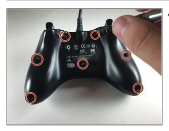
Remove the seven screws from the back of the controller.
