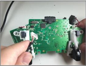
• Remove the wire housing from the opposite side of the circuit board.
