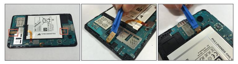
• Using the plastic opening tool, gently pry the chip connections away from the motherboard.
