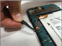
• Using the bent <u>tweezers</u>, carefully pull the flat cables away from the connectors.
