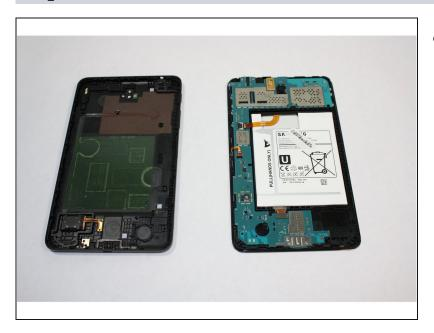
Carefully separate the rear housing from the front panel assembly.
