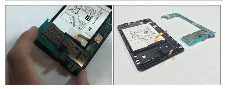
$\triangle$  Use extreme care while removing the motherboard to avoid damaging the component.
