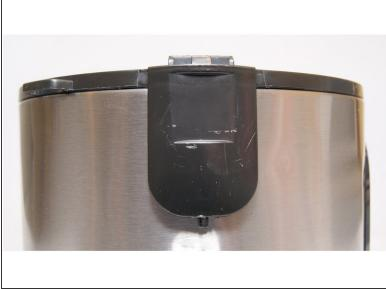
• Locate the piece on the black plastic trim that is opposite from where the hinges were. Carefully, pry the bottom edge of this piece outward (away from the stainless steel side) about 1/4 inch to pull the tab out of it's hole. Once the bottom is pried out a bit, the tab can be seen from the bottom. Press up on the tab with a screwdriver.
