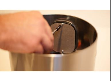
Remove the two screws holding the cardboard cover over the Interface using a Phillips head screwdriver, size PH2.
