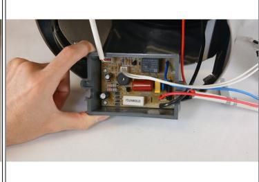
Using a Phillips head screwdriver, size PH2, remove the screws from the control module to expose wired connections.
