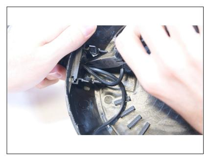
Using pliers, rotate the power cord clockwise to align it with the hole and simply pull it through.
