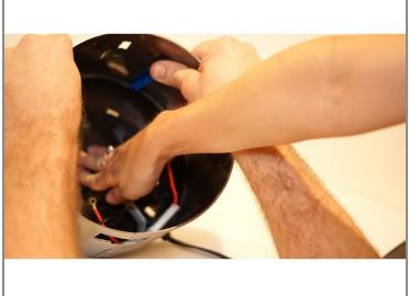
Pry the black base from the stainless steel housing while pushing down on black base from inside the device. This step is much easier with two people. One person can pry while the other pushes.
