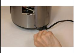
• Locate the hidden screw behind the label and then remove it using a Phillips head screwdriver, size PH2.
