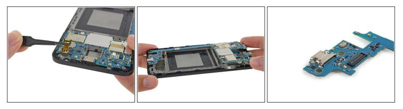
• The 5 MP front-facing camera is the last component preventing us from relieving this phone of its motherboard.
