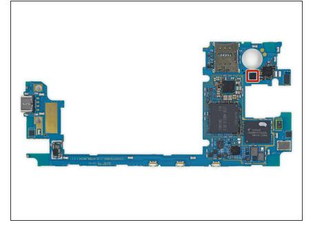
STMicroelectronics <u>STM32F411CE</u> 32-bit 100 MHz <u>ARM Cortex-M4</u> RISC microcontroller
