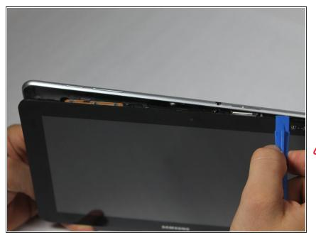
Place your hand between the device and the back panel. Then continue the wedging motion along the top edge of the device until the back panel comes loose.
