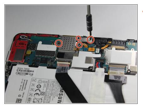
Use a Phillips #00 screwdriver to remove all 4 black 2.5mm screws securing the silver SIM card reader to the motherboard.
