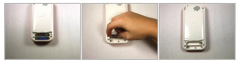
• Remove the two AAA batteries by pulling on one end of the battery and lifting it straight out.
