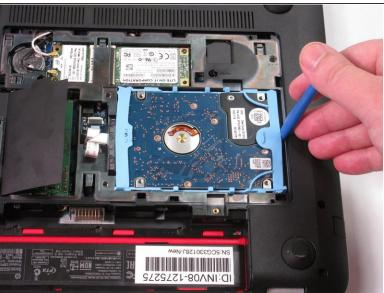
Use the plastic opening tool to pry the hard drive away from the board. Notice that there is a slit centered at the back of where the hard drive is sitting. This is where you'll insert the plastic opening tool as shown in the photo. Finally, pry with the plastic opening tool to remove the hard drive.
