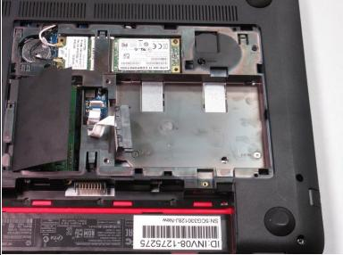
Firmly grasp the connector's base as shown and pull to remove from the hard drive.
