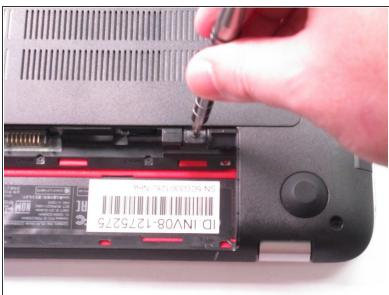
Remove the single screw holding the accessory plate. This is a PH0 2.0x2.5 screw.
