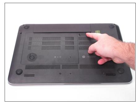
Press the battery release tab and the battery will pop up.
