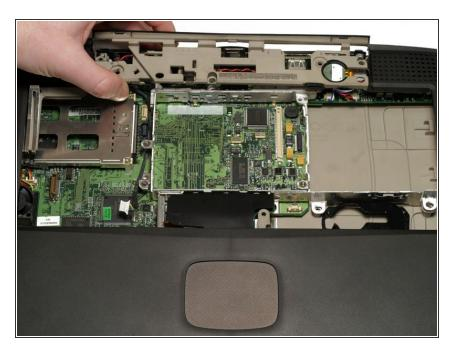
Remove the upper casing. Note that there are two tabs on the laptop's front that often cause the upper case to stick.
