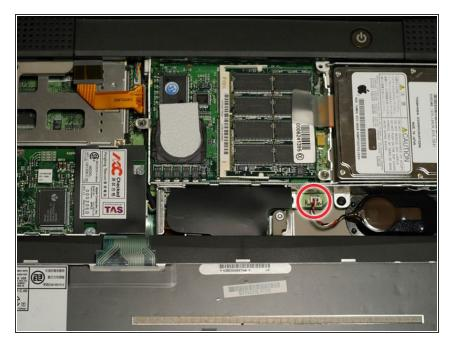
Pull the battery cable directly up from the logic board.
