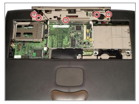
Remove the three long silver and two short black Torx screws from the beige plastic casing.
