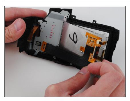
The LCD screen can now be lifted from the right side to be replaced.
