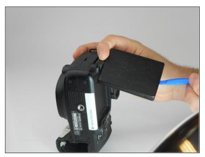
Using a plastic opening tool, carefully pry off the back cover of the LCD.
