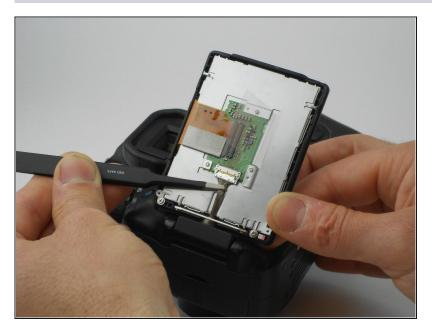
Using the <u>tweezers</u>, carefully disconnect the rear connector by pulling it away from the screen.
