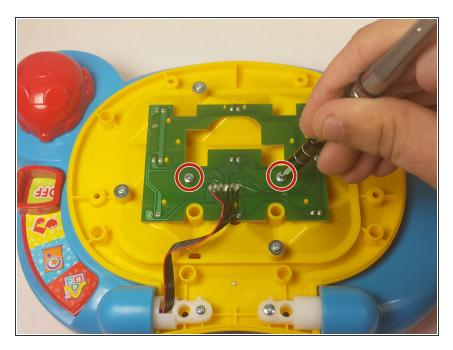
Remove two 6.0mm screws from the LED array using a Phillips #0 screwdriver.
