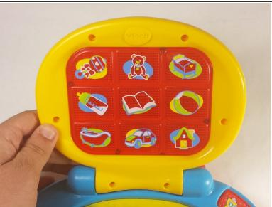
Using a Phillips #0 screwdriver, unscrew the six 7.3mm screws holding the screen together.
