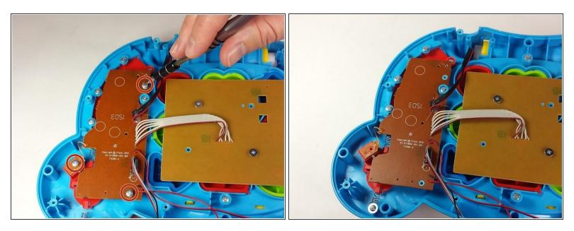
• Using a Phillips #0 screwdriver, remove the three 7.3mm screws.
