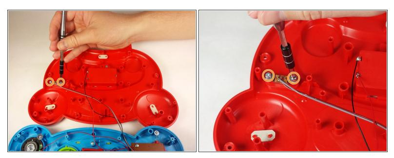
• Use a Phillips #2 screwdriver to remove the two 7.7mm screws on the volume switch.
