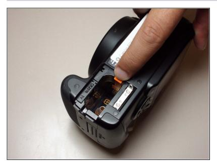
Pull the orange tab to the right to release the primary battery.
