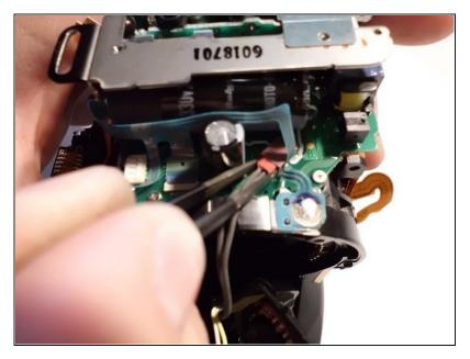
Disconnect the red connector located by the USB port.
