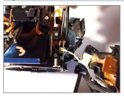
Unplug the yellow connector located on the top of the camera.
