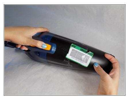
Pull the black nose off of the body of the vacuum, by pushing in the orange button closest to the nose.
