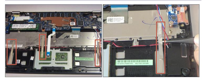
• Use a pair of <u>tweezers</u> to peel up one side of each of the 3 pieces of tape that cover the speaker wires.
