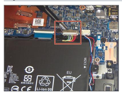
Use a pair of <u>tweezers</u> to gently disconnect the battery connector.
