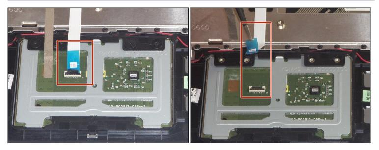
• Use a pair of tweezers to disconnect the <u>ZIF connector</u> securing the trackpad ribbon cable. Gently lift the black tab up, and the cable should come free.
