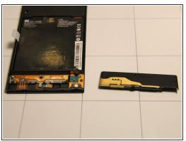
Remove the plastic cover on the bottom of the back panel by inserting the pry tool at the edge and gently lifting.
