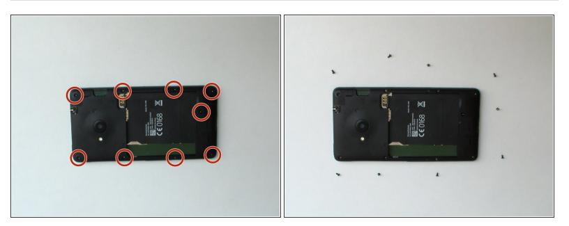
• With a screwdriver Torx T4 remove the 9x screws.
