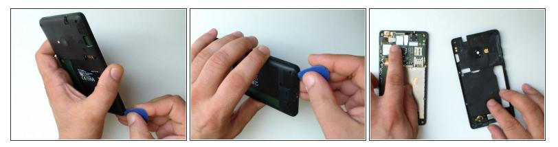
With a plastic opening tool separate the back cover from the middle frame.
