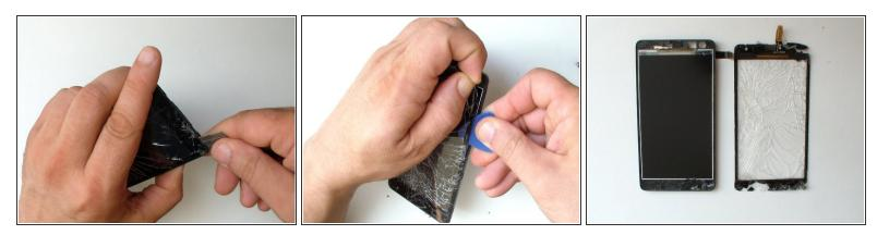
• Use a cutter or other tool with a sharp edge and start the separating from the bottom side. When you make enough room, continue the operation with a plastic tool.
