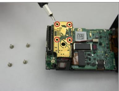
Remove the four 8 mm Phillips #000 screws securing the camera sensor assembly.
