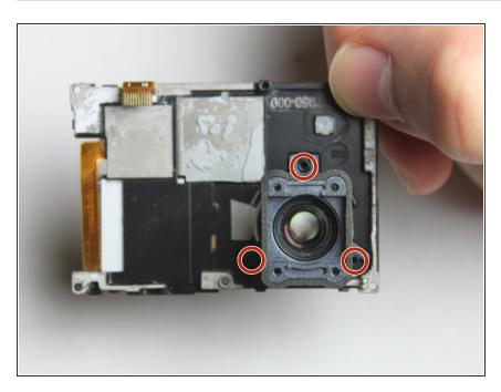
Remove the three 8 mm Phillips #000 screws securing the lens.
