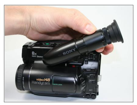
Twist the eyepiece counterclockwise until it stops.
