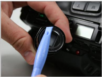
Using the Small Plastic Opening tool, pry the tab on the plastic lens away from the viewfinder.
