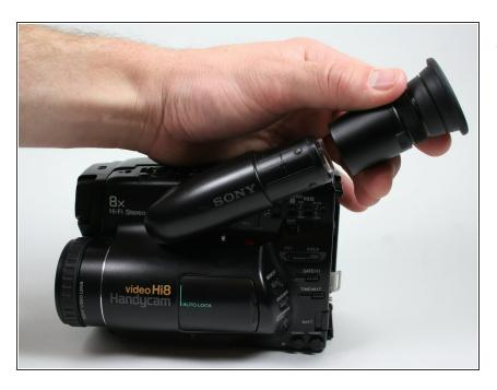
Pull the eyepiece completely off away from the rest of the viewfinder.
