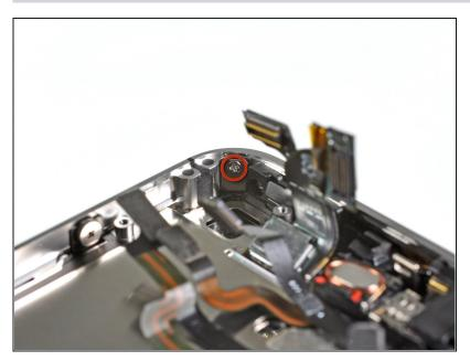
Remove the 1.6 mm Phillips screw securing the display assembly near the power button.
