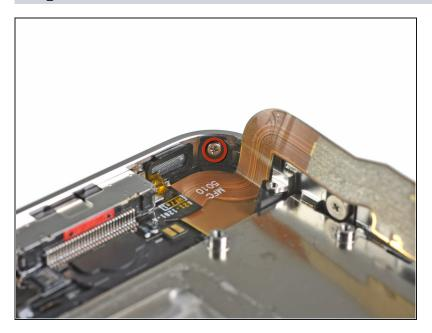
Remove the 1.6 mm Phillips screw near the dock connector cable.
