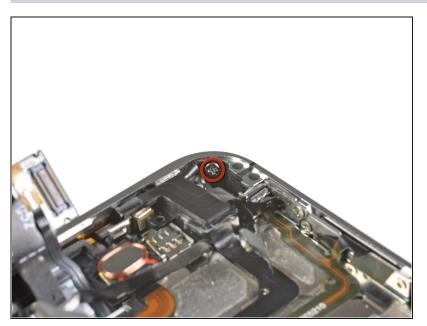
Remove the 1.6 mm Phillips screw near the headphone jack.
