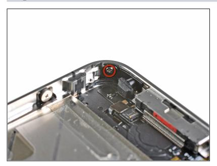
Remove the 1.6 mm Phillips screw near the lower microphone.
