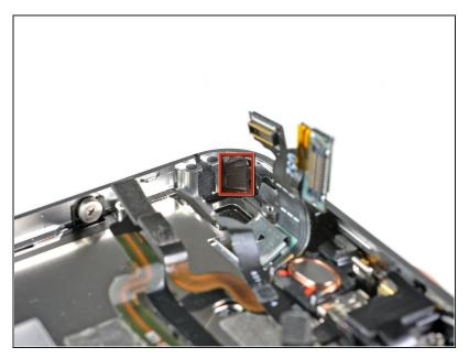
Remove the small pieces of black tape covering the display mounting tabs.
