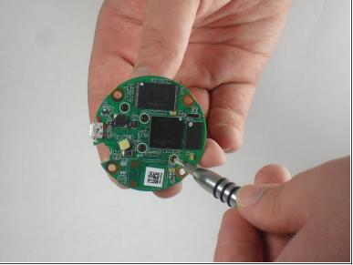
Using a Philips #0 screwdriver, remove the four 2 mm screws.
