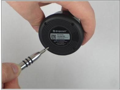
Using a Philips #0 screwdriver, remove the four 3 mm screws.
