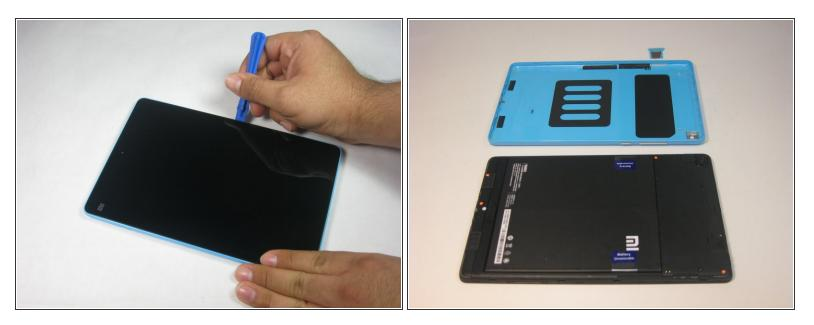
Use a plastic opening tool and/or opening pick to gently pry the back panel away from the device.
