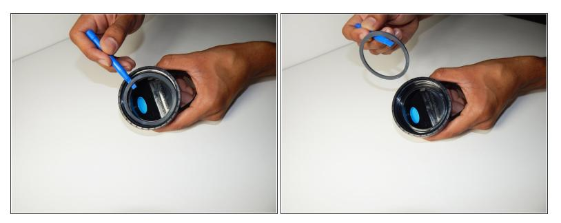
Gently pry the seal up while lifting seal out of the seal seat.
