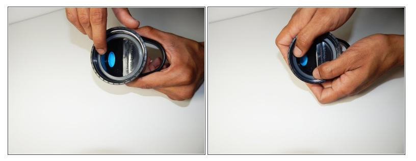
Press new seal into seal seat with finger.
