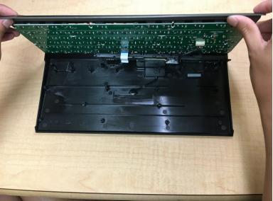
Carefully separate the bottom half of the keyboard from the top half of the keyboard.
