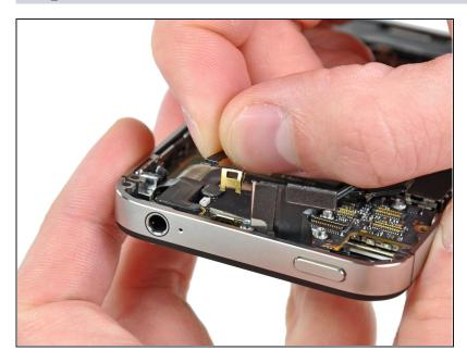
• Lift the small grounding clip up off the logic board and remove it from the iPhone.
