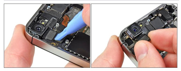
• Use the edge of a plastic opening tool to pry the rear camera connector up from its socket on the logic board.
