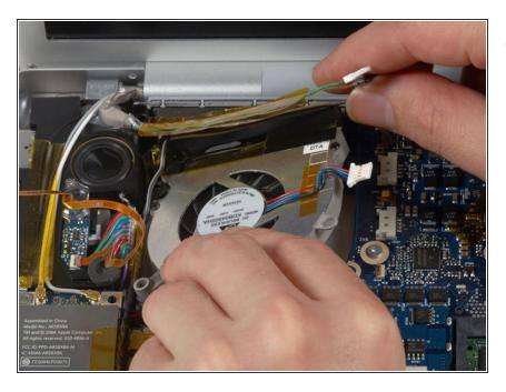
Lift the lift fan up and carefully peel up the tape securing the fan to the heat sink as you go.
