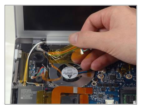
Peel up the iSight and inverter cables from above the left fan, removing tape as necessary.
