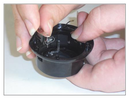
• Lift the mounting clips away from the case.
