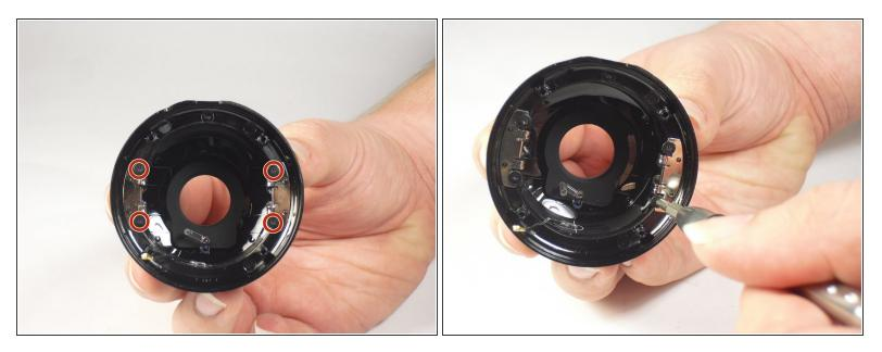
Using a Philips #0 screwdriver, remove the four 4 mm screws that are attaching the mounting clips to the case.
