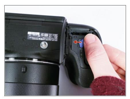
Push the blue tab that secures the battery. The battery will then spring out.
