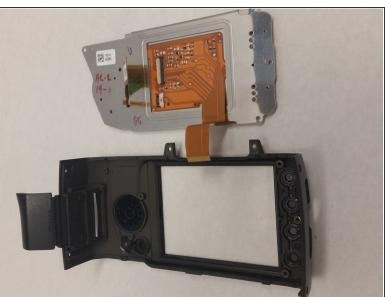
Remove six 5 mm x 4mm Phillips head screws, then remove the metal plate housing the LCD from the plastic camera backing.
